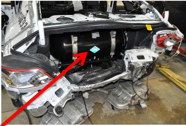
Post-test photo shows CNG tank integrity
